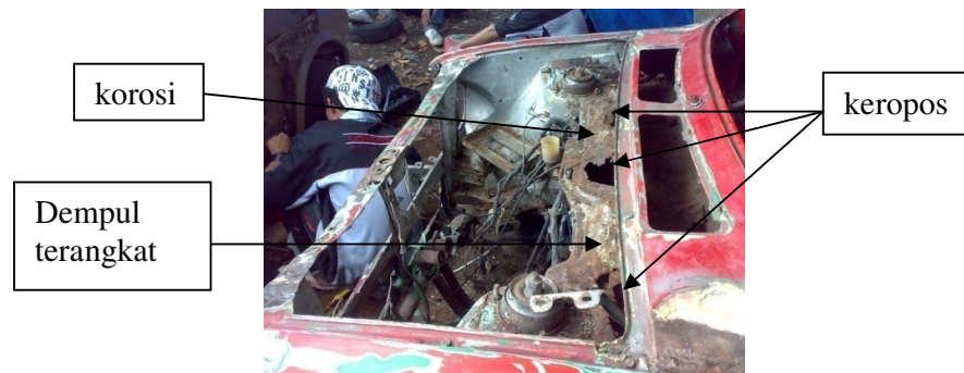
Gambar 67. Kerusakan bagian dash board panel
