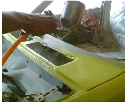
Gambar 72. Proses pengecatan dasar ( under coat )
