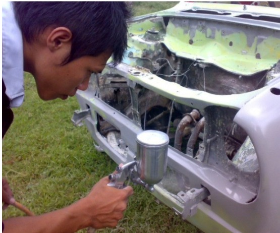
Gambar 71. Proses pelapisan surfacer
