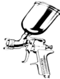
Gambar 19. Spray gun tipe gravity feed (Gunadi, 2008:457)
