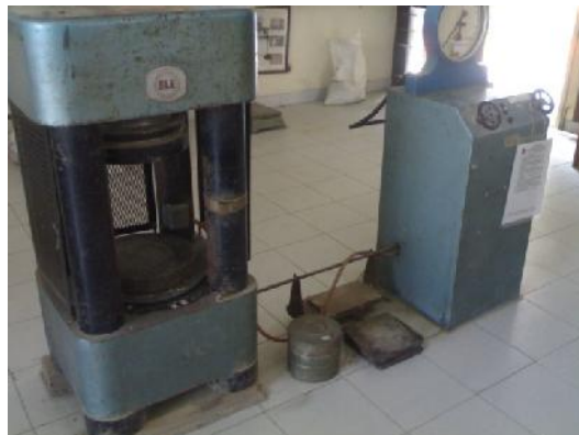
Gambar 37. Compression testing machine (CTM)
