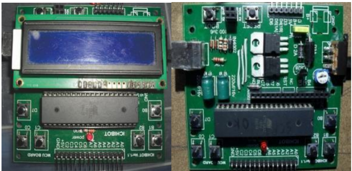
Gambar 26. Realisasi PCB Microcontroller Unit (MCU)
