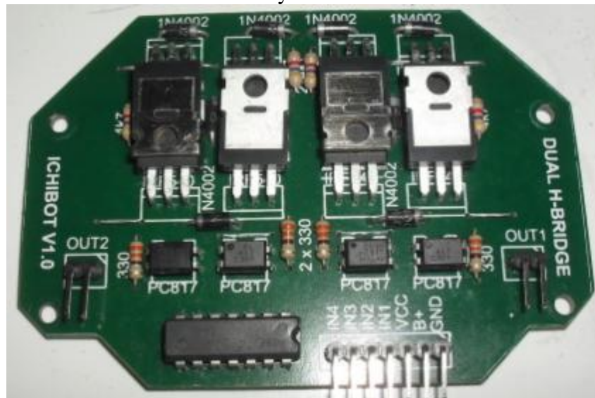
Gambar 29. Layout PCB Driver Motor
