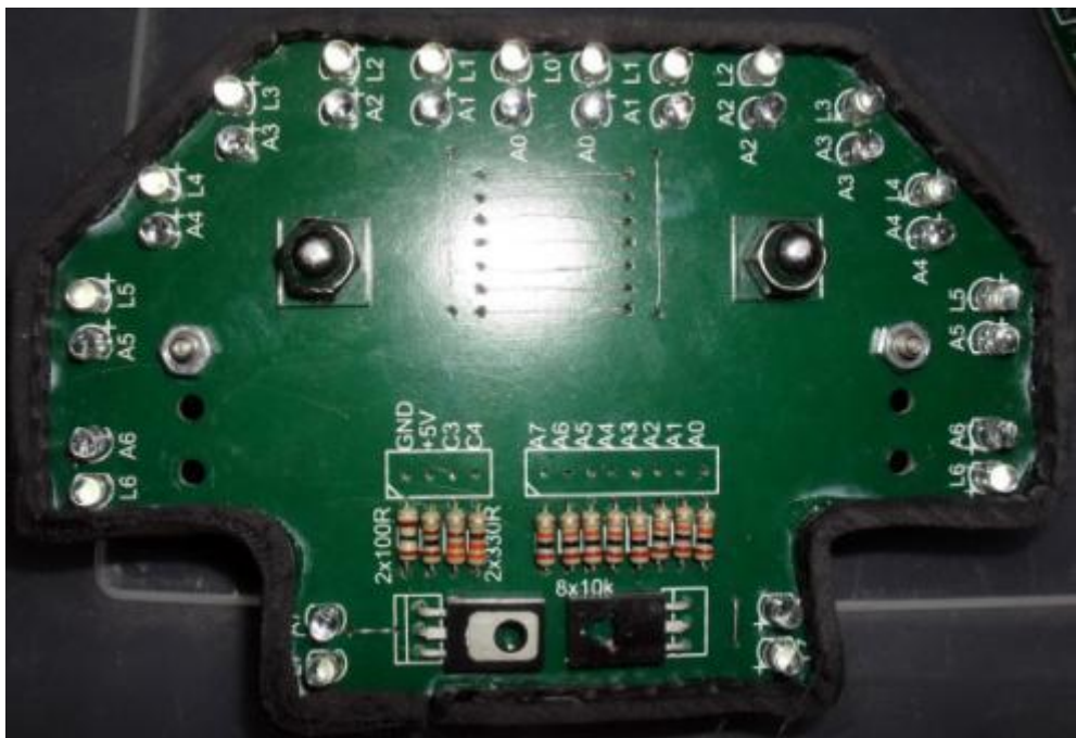
Gambar 27. Layout PCB Line Sensor (Sensor Garis)
