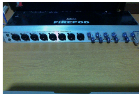
Gambar 3: Sound card External Fire Wire ( Dok : agung , Maret 2013 )
