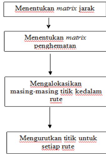
Gambar 2.3 Skema metode saving matrix
