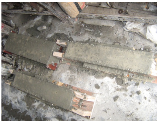
Foto 12. Mencetak campuran beton Hybrid Fiber Reinforced Self-Compacting Concrete (HyFRSCC)
